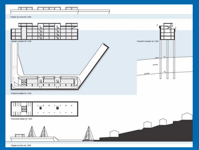
Due to the great sea depth and exposure of the location to wind strikes, the breakwater must be constructed. This will be done in the way to form 20 meters wide semi-submerged structure within the primary breakwater. Therefore, besides giving proper protection against bad weather, it could serve as a structure for the placement of various attractive and necessary contents of the 5-anchor marina on the gross developed surface of approximately 7.000 m2 on each of 5 floors
